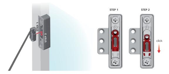
Lift the door almost completely to slot the end element of the wire into the door bracket.
