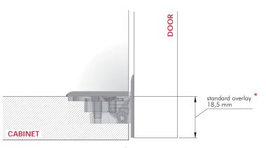
\* this dimension can be changed by modifying the drilling plane or by using the spacers.
